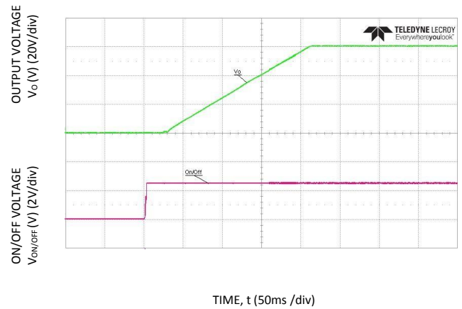
Figure 14. Typical Start-up Using On/Off Voltage (V IN = 48V, I o = I o,max ).
