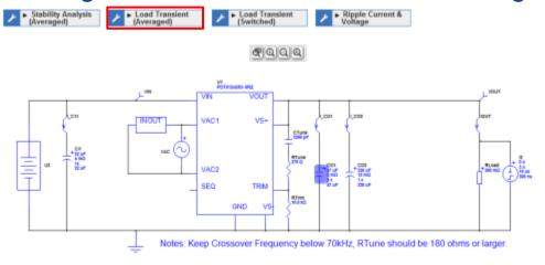
Check pk-pk value of Vout is below design requirement of 25mV by selecting PK-PK from the measurement drop down menu.
