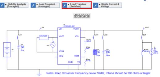
Check pk-pk value of Vout is close to design requirement of 25mV by selecting PK-PK from the measurement drop down menu.
