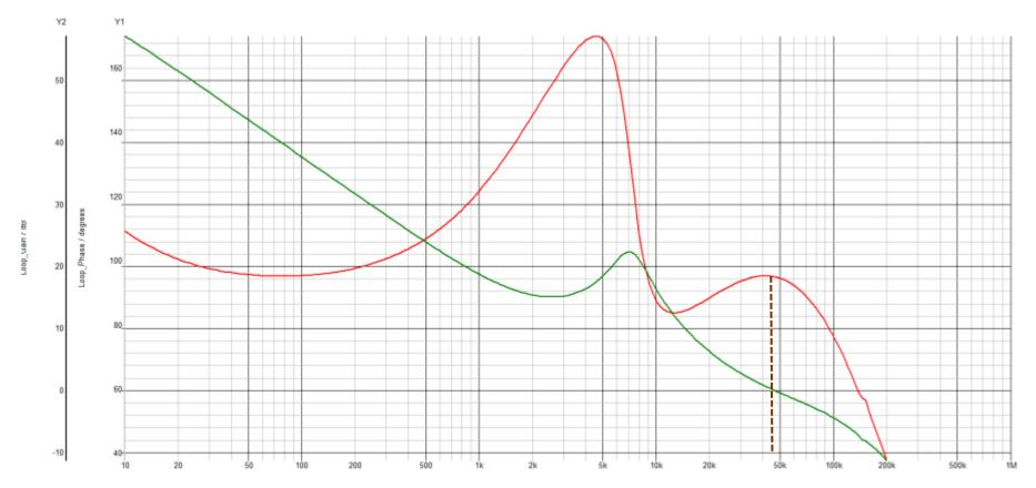
The values of crossover frequency and Phase Margin are close to the values of 46kHz and 95degrees from the online tool
