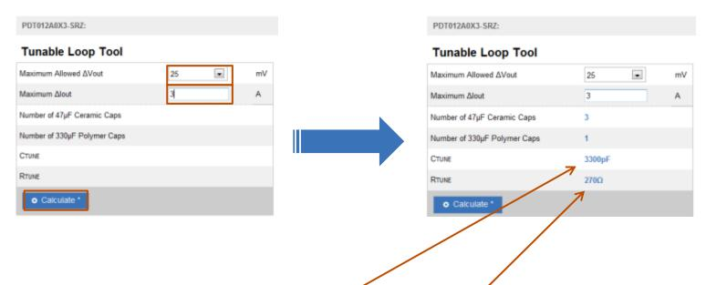
• The tool provides the Ctune and Rtune values to achieve the desired Δyout.
