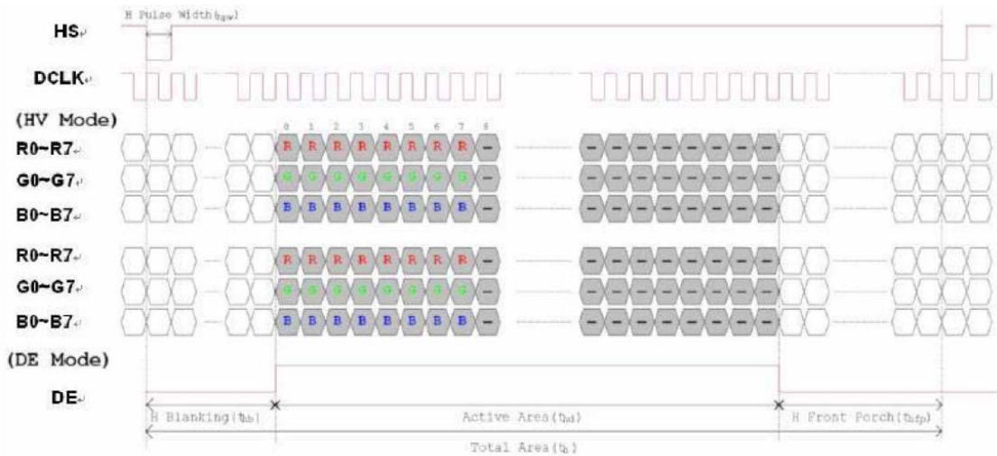
1 Horizontal input timing diagram.
