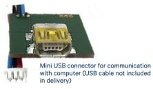
Serial interface connector to SiPM Module
